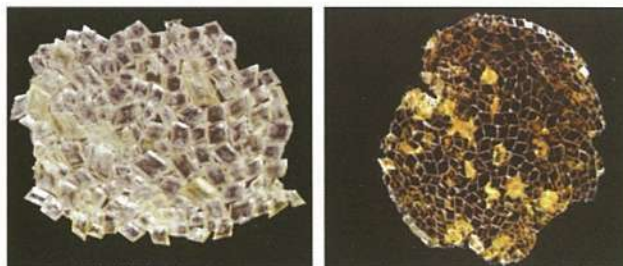
Figure 12. Photographs of white crusts and yellow crusts of glycine crystals grown at the air/aqueous solution interface in the presence of N ε-(2,4-dinitrophenyl)- S -lysine and leucine in a ratio S/R > 1 and S/R < 1 , respectively. The white crystals exposed their (0 \bar{1} 0) face towards the solution whereas the yellow crystals exposed their (00) face.
