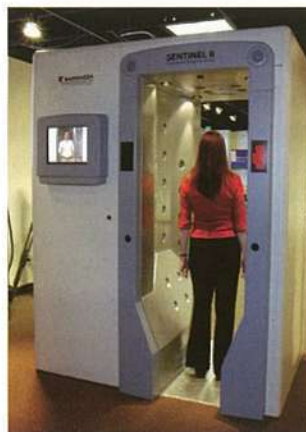
Figure 4: Ionscan Sentinel II, Commercialized Version of Explosives Detection Personnel Portal with IMS Detection, developed by Smiths Detection and Sandia National Laboratories. (Photo by Sandia National Laboratories – used with permission).
