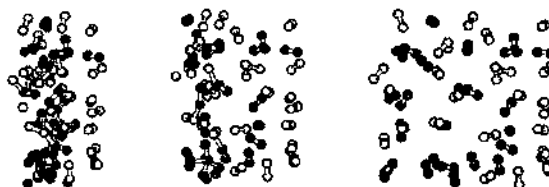
Figure 2. Configuration of O and N atoms at three different times during the compression stage of a cluster of 30 O 2 and 30 N 2 molecules. The wall, not shown, is at the left and the impact velocity is 12 kms -1 . Note the formation of NO and of transient polymers.
