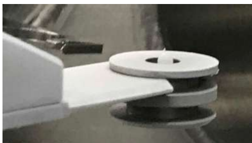
Figure 1: Frozen liquid sample in the loading compartment of the XPS instrument.
